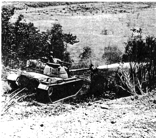
BURN, BABY, BURN-- A Marine tank driver burns brush to clear a road shoulder along Rt #9.
