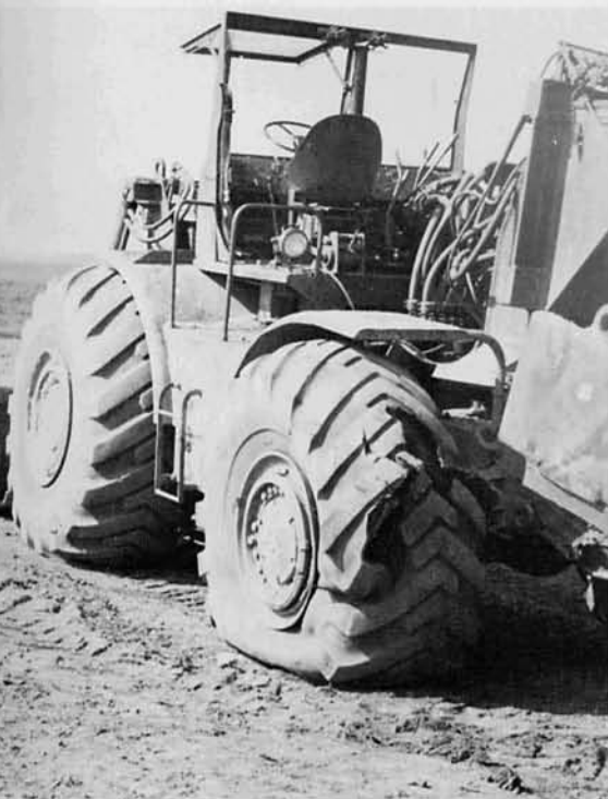
The tire of this MRS had a chunk blown out of it by a Viet Cong land mine while working at the Gia Lo rock quarry.
