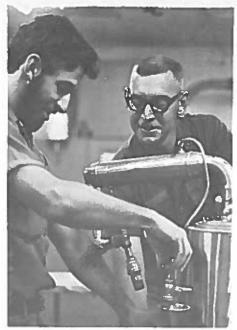
CE3 John Miller and CE1 Ray Winstead (shop supervisor) work on a distilling unit that provides pure water for TIG welding machines.
