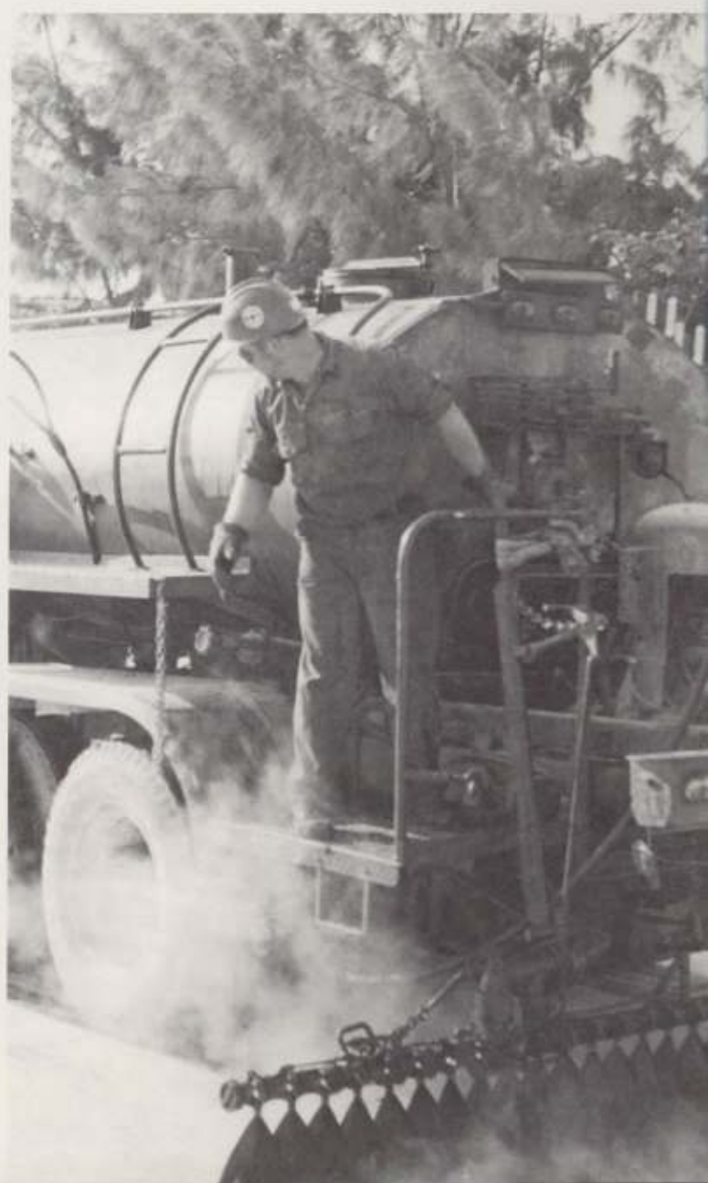
EO2 Daniel Smith operating the rear end of an asphalt distributor.
