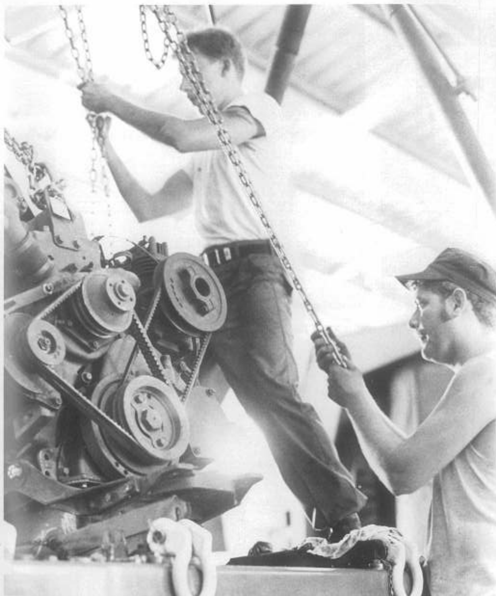
CMCR Kent and CM3 Bridges replace engine in Five-ton.
