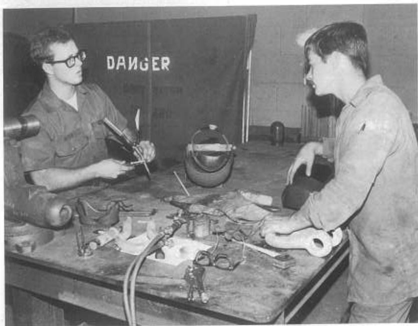
EO2 Nelson and SW3 Anderson repair honing tool.
