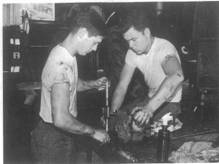
CMCN Huck and CMCN Carper tap out holes on hydraulic transfer pump.
