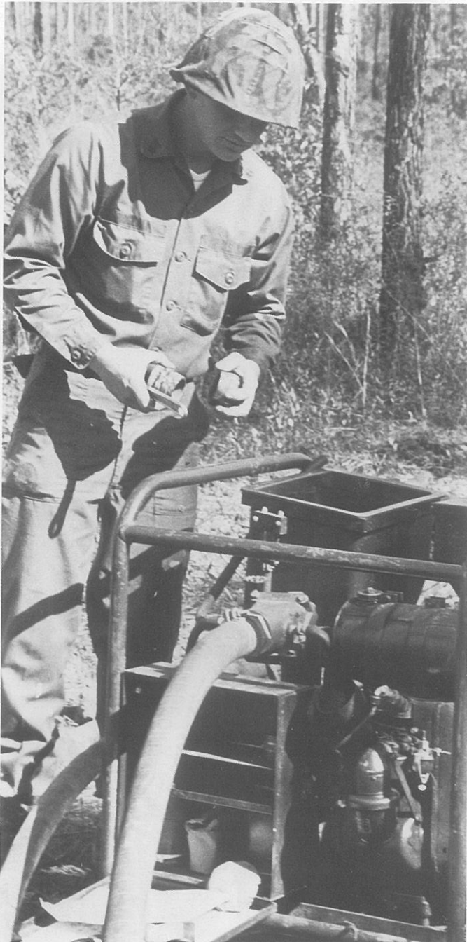
UT2 Bruce Ridgeway works on the ND-25 Water Purification unit.
