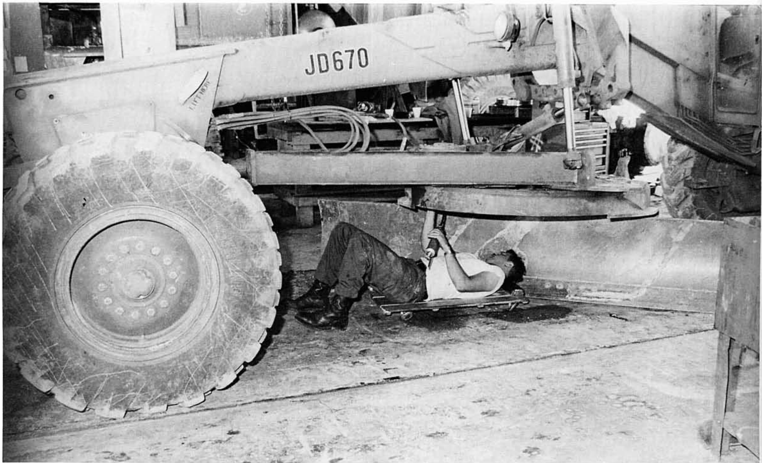
CMCN Rusty Shook isn't trying to catch a nap. He's doing preventive maintenance on a grader.
