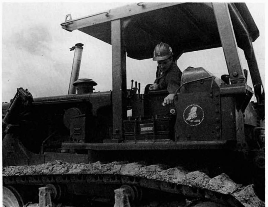
CM3 Clifford Blake checks the fluid level in the battery.
