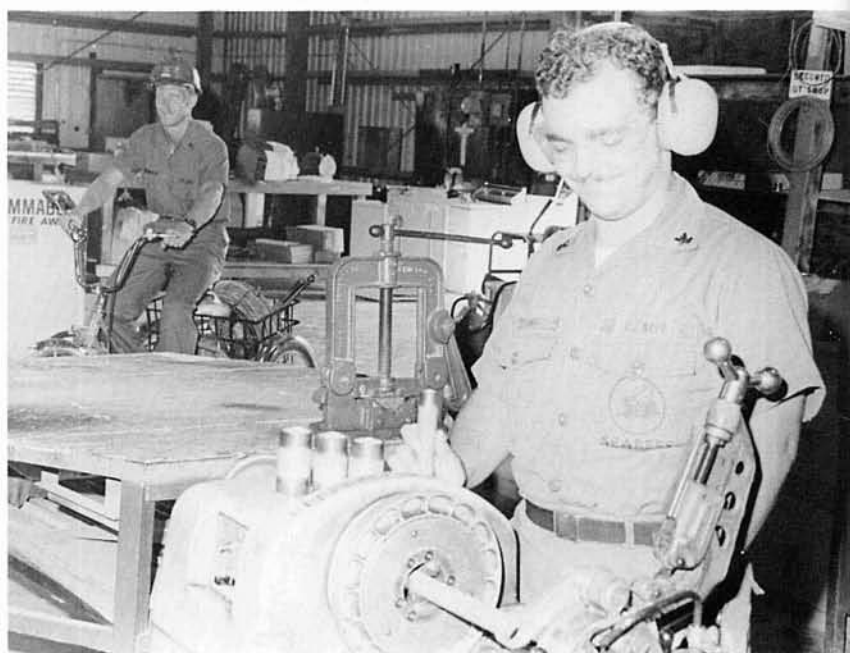
UT2 Scott Mowrer returns from his rounds as UT2 Gary Stumpf threads pipe.
