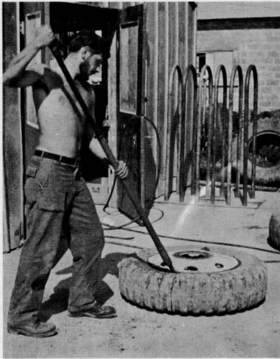
NEW RUBBER --Construction Mechanic Apprentice H. E. Webster changes a tire on a wheel off a five-ton truck at the automotive shop.
