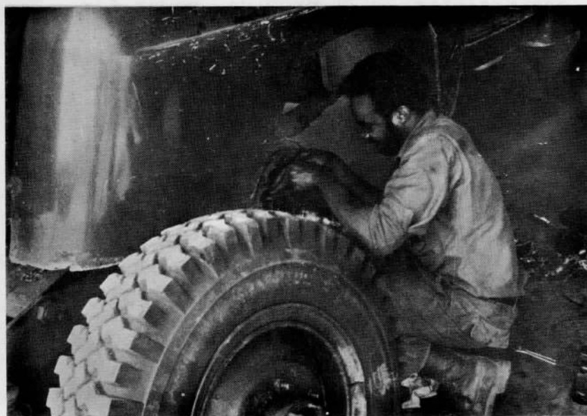
NEW SHOES--Construction Mechanic Third Class Thomas West replaces the brake shoes on a one-ton truck at NMCB-62 automotive shop at Camp Moscrip.
